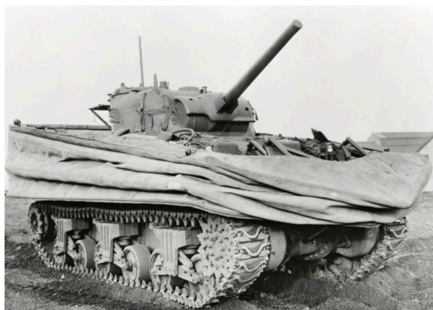
Sherman DD tank - flotation canvas lowered. Image: IWM MH3660
